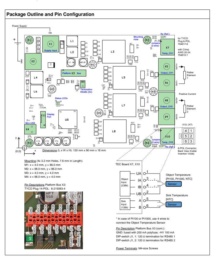
Peltier elements, temperature probes, power supply and connectors not included.
