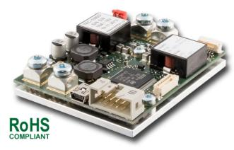
The TEC-1090 is a specialized TEC Controller / power supply able to precision-drive a single Peltier element.
