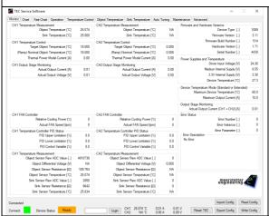
The included TEC Service Software is a powerful tool that allows monitoring, data logging and full configuration of the TEC-1090 via a standard USB or an RS485 connection from a PC running Windows.
