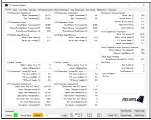
The included TEC Service Software is a powerful tool that allows monitoring, data logging and full configuration of the TEC-1089 via a standard USB or an RS485 connection from a PC running Windows.
