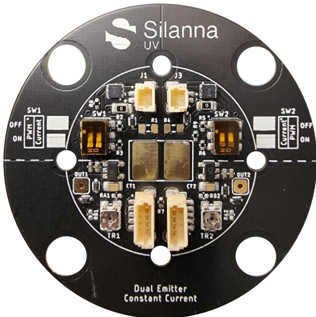
SCC-C50-2ULMS5 Dual Emitter Constant Current Emitter Reference Board
