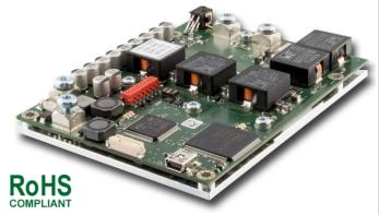
The LDD-1125 is an innovative laser diode driver that contains a specialized current source able to precisiondrive laser diodes in continuous / modulated and pulsed or mixed operation. Equipped with optional laser power measurement circuitry (photodiode input), the LDD-1125-LPC can also be operated as a Laser Power Controller.
