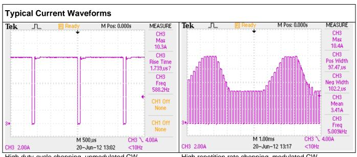
High duty-cycle chopping, unmodulated CW.
