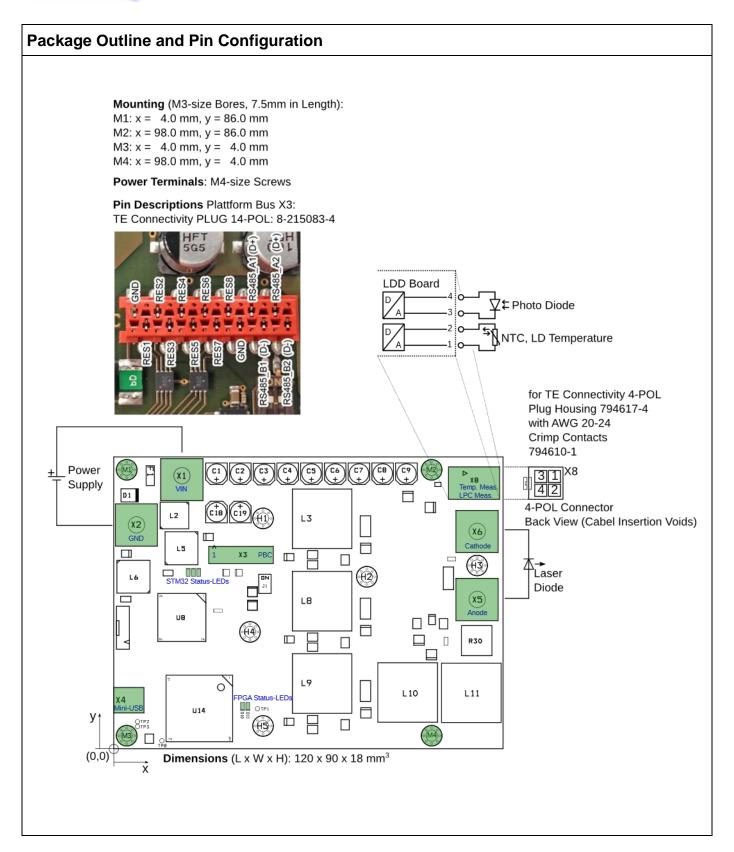
Laser diode, temperature probes, power supply and connectors not included.
