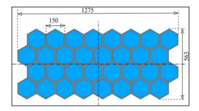
Figure 6: Field-of-View (FoV) Description of the Sensor
