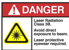
Figure 7: Laser Safety Warning Sign for Unrecommended/Nondefault Operation
