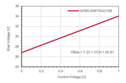
Figure 2: SiPM Bias Voltage vs. Ctrl Voltage
