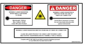
\*Caution: Use of controls, adjustments and procedures other than those specified herein may result in hazardous laser radiation exposure.
